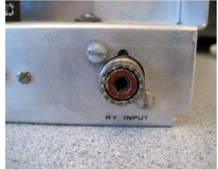
The original RCA plug had been replaced, but the replacement is worn out now.
