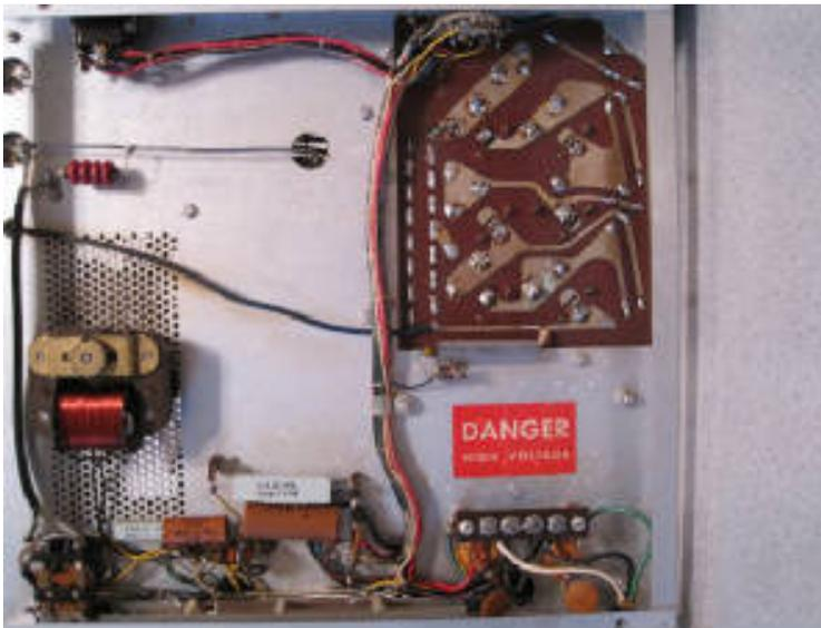
The initial under chassis view with the old HV Power supply in
