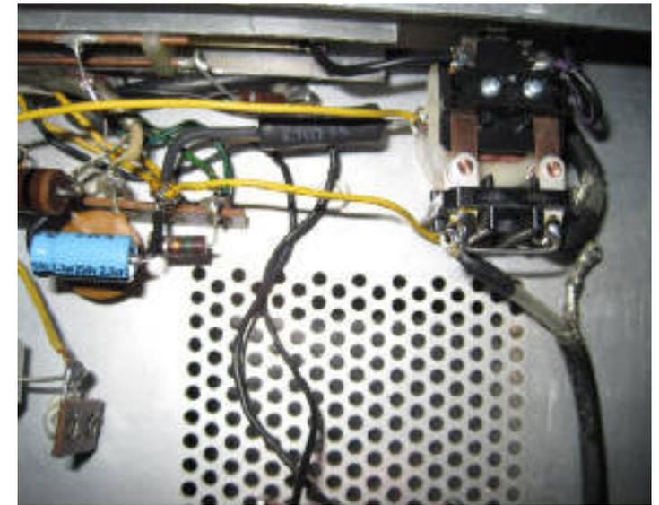
The new Relay was installed with the new resistor for Volt operation. I also replaced the electrolytic caps w units.
