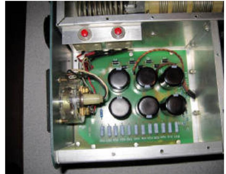
The new HV PCBA in place. The caps are smaller in size with greater values. I added heat-shrink to the transformer leads to help protect the old insulation..
