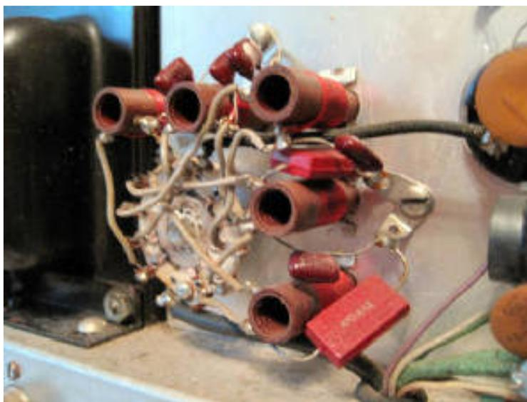
I left the original Exicter Input Section as it was wired when the Amp was built.
