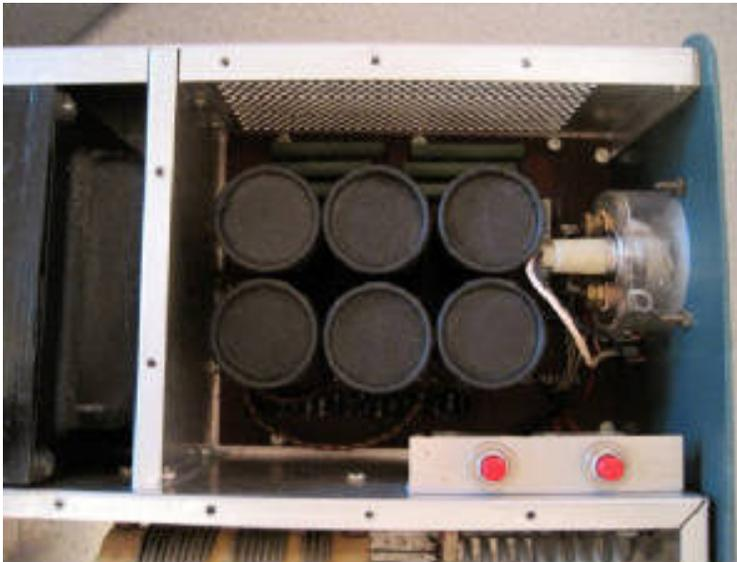
The original power supply with old dry caps and heat stressed components. When I removed it, I unsoldered the meter connections so I did not need to damage the old PCB.
