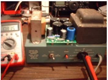
supply produces several medium (-130v, +250, +300 volts) and one high (820 volts) voltages. This project should NOT be taken on without care, planning, and proper tools. There be 800-volt dragons therein. You'll also need to be very familiar with the layout of your variant of the 4 different HP-23 models and whether you'll need the fixed or power-supply adjusted bias.
