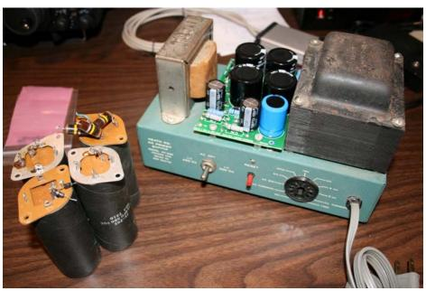
I looked around and found a swell solution that wasn't too expensive. The Heathkit Shop (http://www.theheathkitshop.com/heathkithp-23rl.htm) has an option that replaces the four tall capacitors on the top of the chassis and also all of the point-to-point wiring below with a single PC-board. He sells a complete replacement kit (\$56), but since I have sources locally, I opted for the \$20, PC-board ONLY option.
