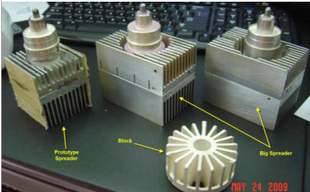
I used the original set of cores and spread the 40m tank over the two sets. Each set is a stack of T200-2. About 2 uH per core for a bit over 4.2 uH. I'm not sure if putting the two cores in series (vs just adding more turns to a single core) helps but it was easy to do.
