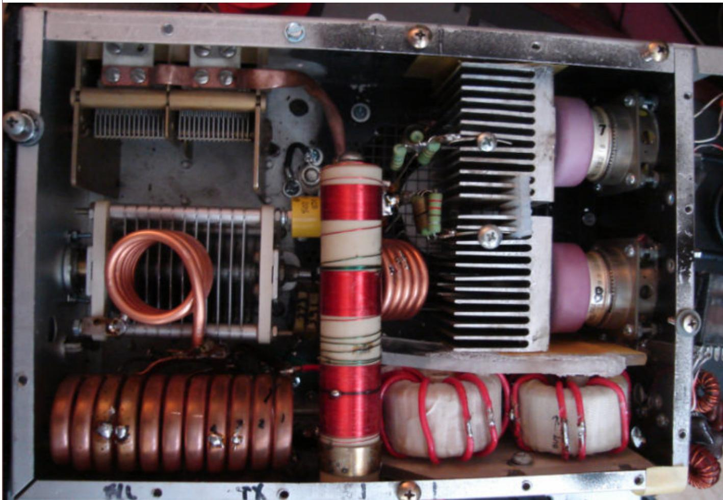
Another check of the amp at full drive levels had the controls (other than tune on 15m) away from the stop. And efficiency at 61% 40m, 62% on 20m and 57% on 15m. This is a big step up from 45%/55%/50% level before the change. And that shows the amp running around 1KW out while staying within the official plate dissipation limits (700w).
