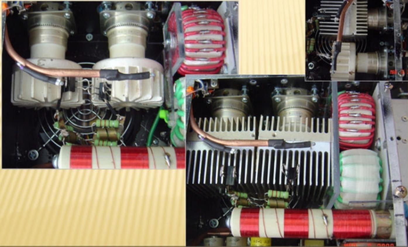
After getting a couple of iterations of spreaders built, I knew the tank was thrown way off on the higher bands. But this was a couple of years ago and 20m was the only usable higher band. Things have changed now and my prior patch of just dropping the tank's L with some shorting here and there on coils was coming back to haunt me. Very high Q, and with that a lot of dissipation both in the tank and probably in the tubes as well.
